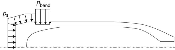
FIGURE 4.16 Load conditions for an M1 HE projectile.
