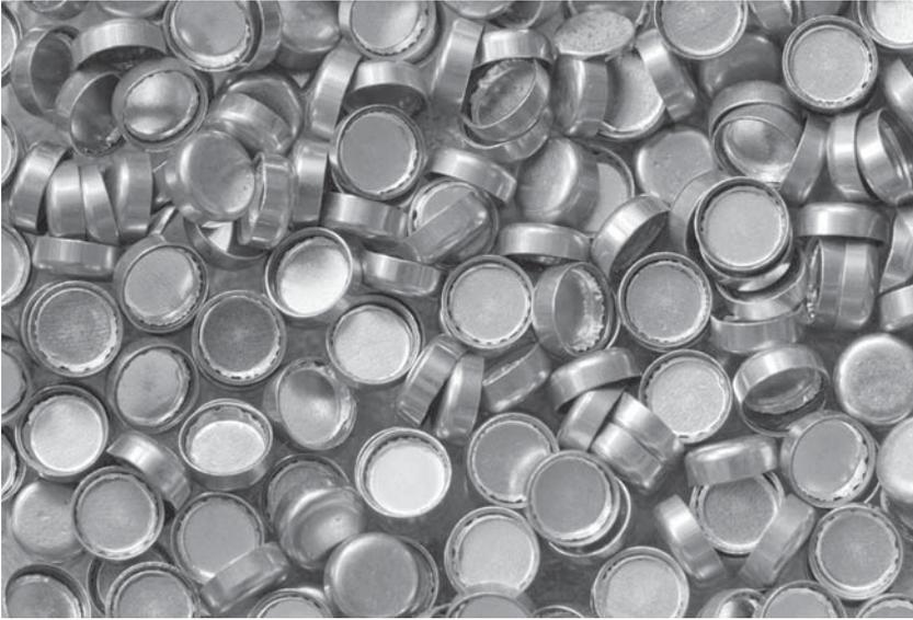
The primer is the component contained and held in the center of the base of the metallic cartridge case. It contains an explosive compound. When struck on its metal side by the firing pin in your gun, it will ignite the powder sitting in front of it within the case, building up pressure to send the bullet out of the case, down the barrel, and out to your target.
